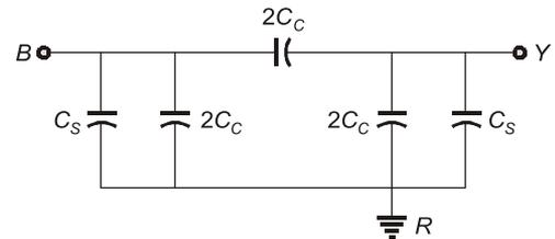
$$C_{BY} = \frac{C_s + 2C_c}{2} + 2C_c = \frac{C_s + 6C_c}{2}$$
